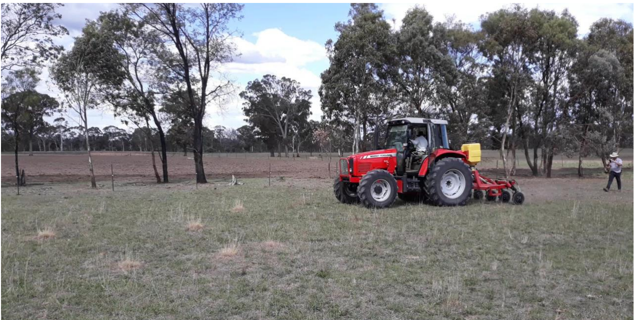
Figure 5. A low disturbance planter fitted with an in-furrow liquid inject system for applying bio-stimulants while planting [Photo: Lee Fieldhouse].
