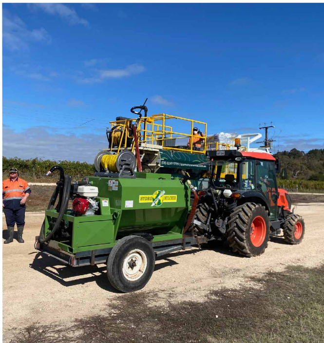
Figure 11: LCS Environmental hydroseeding equipment in autumn 2025 [Photo. Nathan Foreman].
