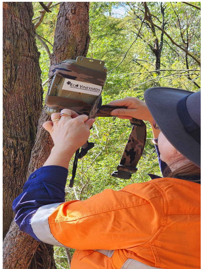
Figure 5: Installing chorus detector for microbat echolocation signal monitoring [Photo: Melbourne Water].
