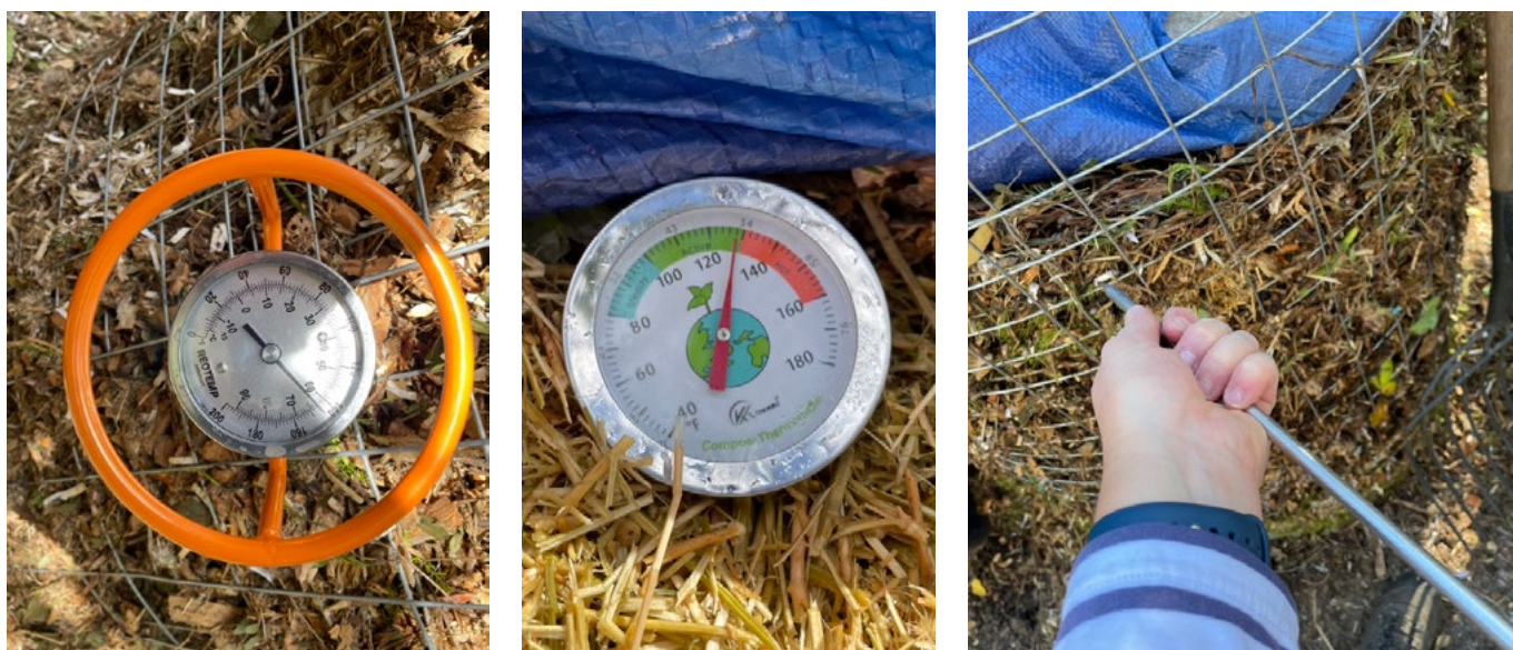
Figure 7. Compost thermometers that are purpose designed to keep a close eye on temperatures of the compost pile [Photos: Mary Retallack].
