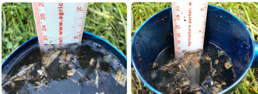
FIGURE 17: Measuring the water infiltration rate over a 6-minute period [Photos: Mary Retallack]
