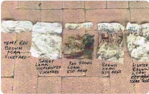
FIGURE 9: Installed in August and retrieved in September (6 weeks) in different soil types [Photo: Mary Retallack (left) Peter Freckelton (right)]
