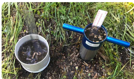
FIGURE 16: A water infiltrator made from PVC pipe (left) and stainless-steel soil water infiltrator (right) [Photo: Mary Retallack]
