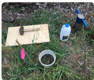
FIGURE 15: Installing a water infiltrator [Photos: Mary Retallack]
