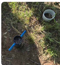
FIGURE 15: Installing a water infiltrator [Photos: Mary Retallack]
