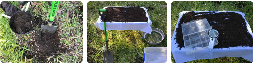
FIGURE 6: Assessing soil macroorganisms in the field. Soil reducer (left), spade, 10mm sieve and folding table with white cloth (centre), sample ready for assessment with a collection container and handheld magnifier (right)
