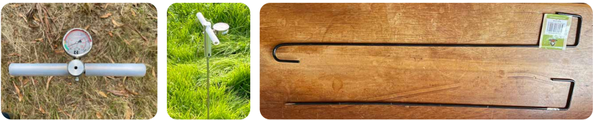
FIGURE 13: Soil penetrometer (left and middle) and home-made soil penetrometer (right) [Photos: Mary Retallack]
