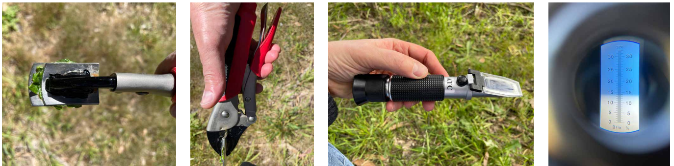
Figure 5. Leaf Brix can be measured using a pair of modified vice grips to extract leaf sap and a refractometer which provides an objective measure of plant health [Photos: Mary Retallack].
