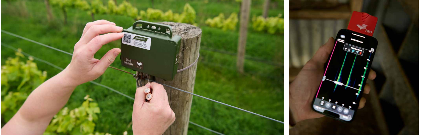
Figure 4. Examples of devices used to detect microbat activity, including Wildlife Acoustics Song Meter Mini Bat (left), and Wildlife Acoustics Echo Meter Pro 2 attached to a mobile phone (right) [Photos: Colin Page].
