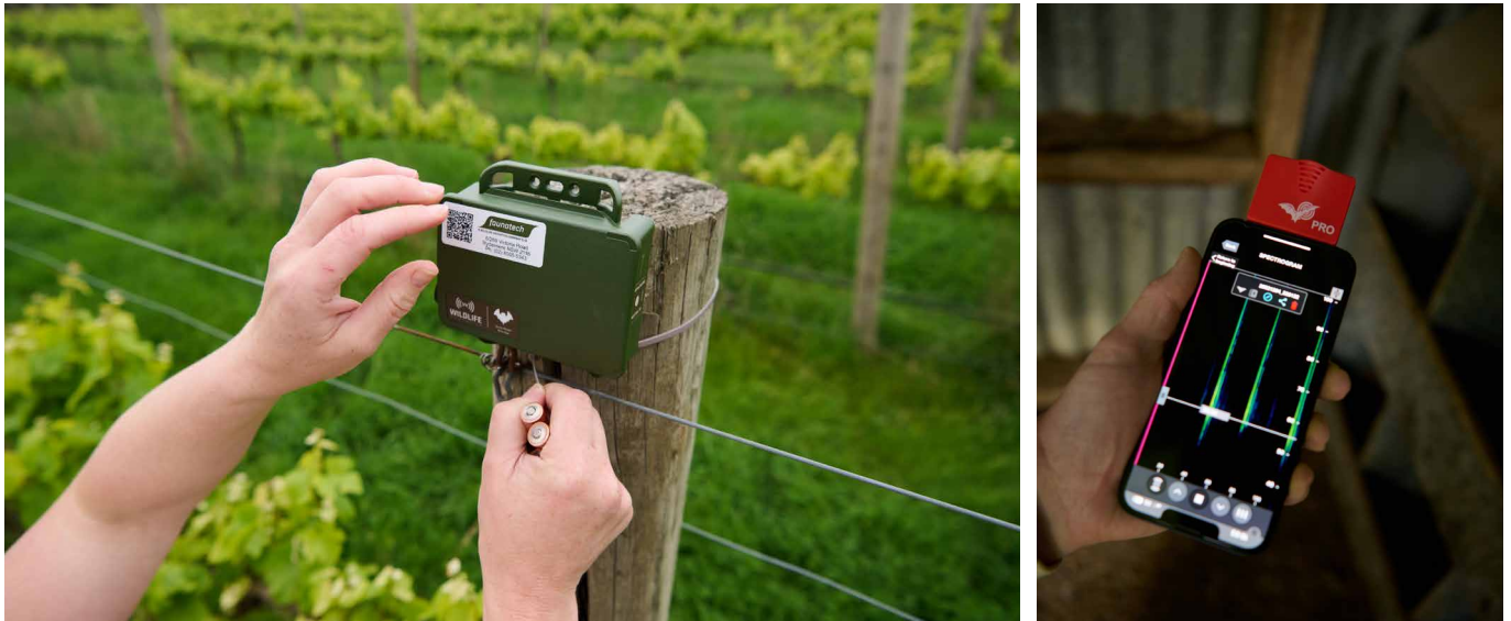
Figure 4. Examples of devices used to detect microbat activity, including Wildlife Acoustics Song Meter Mini Bat (left), and Wildlife Acoustics Echo Meter Pro 2 attached to a mobile phone (right) [Photos: Colin Page].
