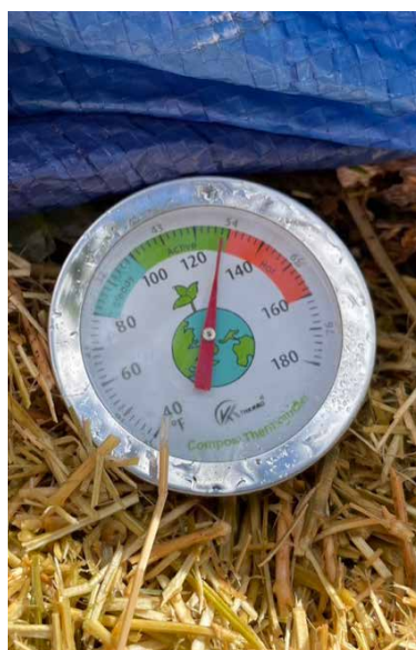
Figure 7. Compost thermometers that are purpose designed to keep a close eye on temperatures of the compost pile [Photos: Mary Retallack].
