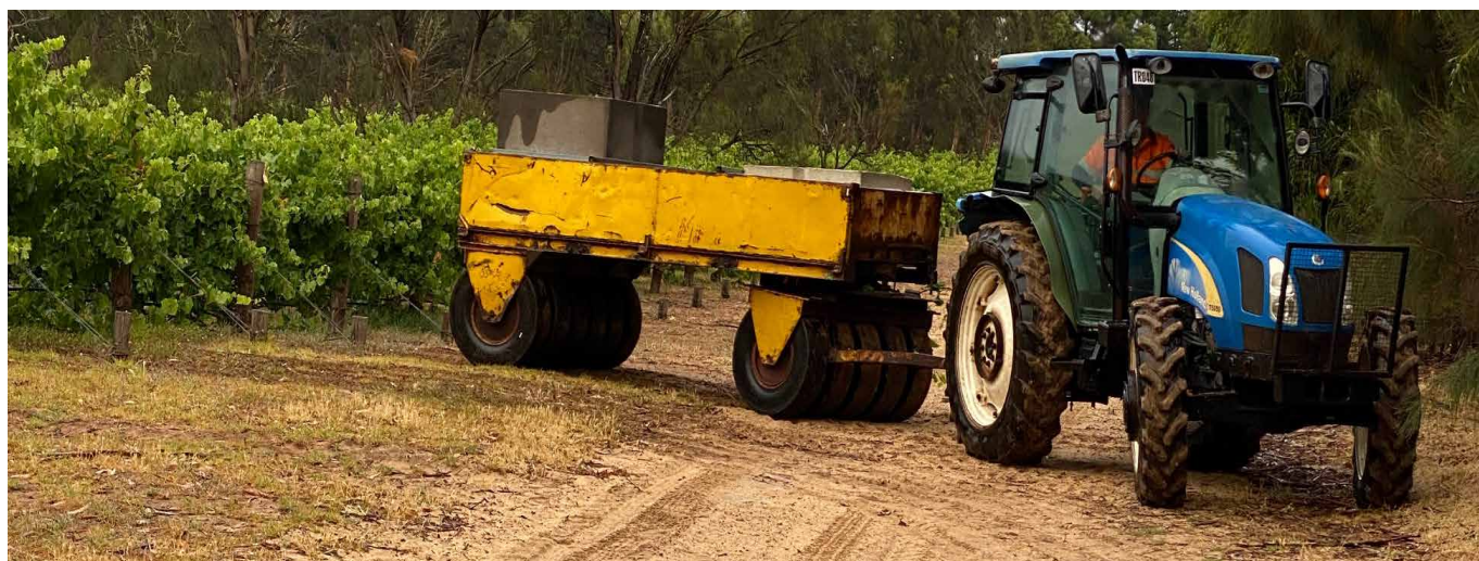
Figure 8: Snail roller used at Guichen Bay and Wrights Bay Vineyards, Mount Benson, SA [Photo: Dean Barker].
