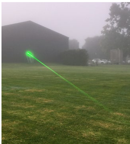
FIGURE 48. Some bird control devices use a focused green laser beam to deter birds from specific areas [Photo: Phil Barron].
