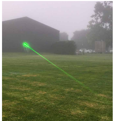
FIGURE 48. Some bird control devices use a focused green laser beam to deter birds from specific areas [Photo: Phil Barron].
