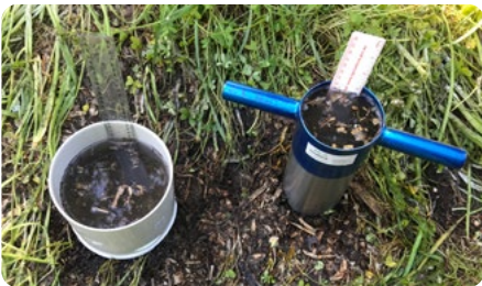
FIGURE 14: A water infiltrator made from PVC pipe (left) and stainless-steel soil water infiltrator (right) [Photo: Mary Retallack]
