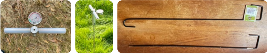
FIGURE 11: Soil penetrometer (left and middle) and home-made soil penetrometer (right) [Photos: Mary Retallack]
