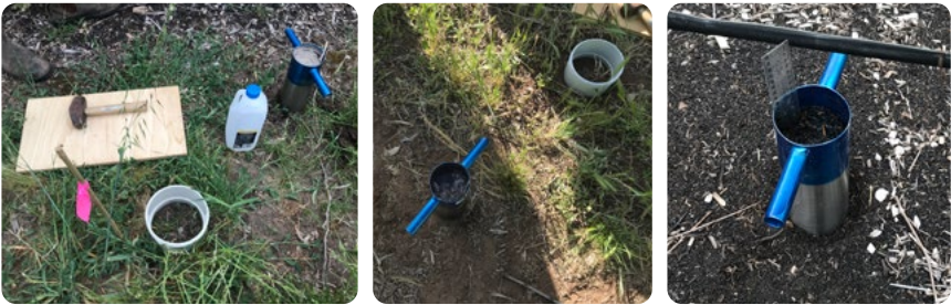
FIGURE 13: Installing a water infiltrator [Photos: Mary Retallack]
