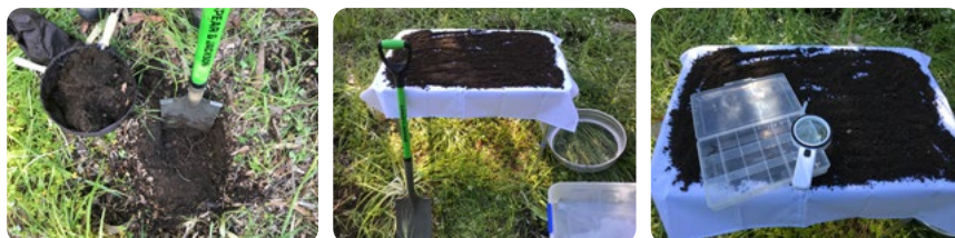
FIGURE 5A: Assessing soil macroorganisms in the field. Soil reducer (left), spade, 10mm sieve and folding table with white cloth (centre), sample ready for assessment with a collection container and handheld magnifier (right)
