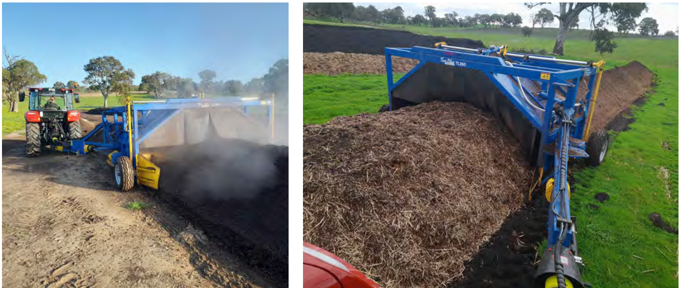
Figure 21. Turning compost windrows with a specialised compost turner [Photos: Dan Falkenberg].
