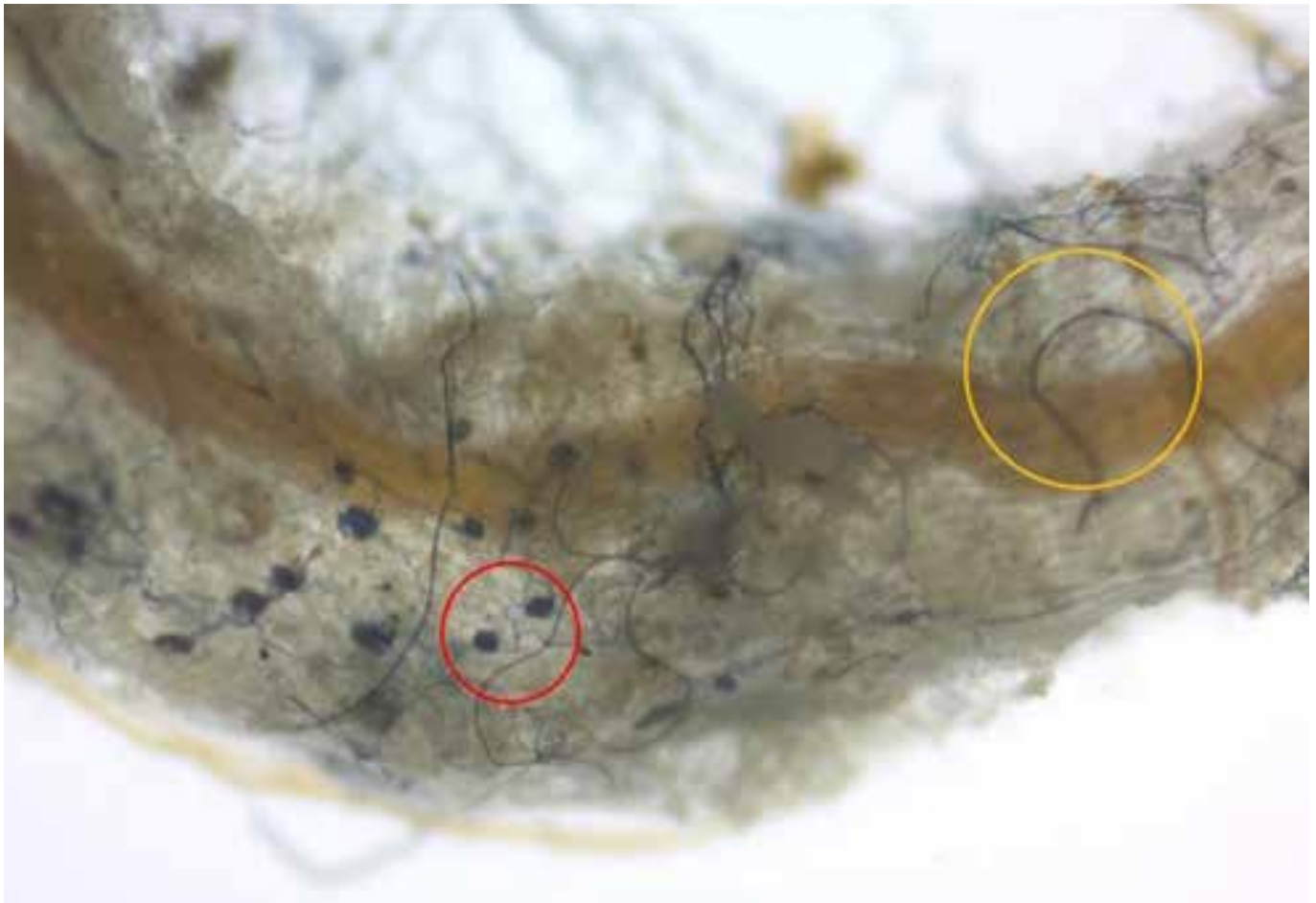
Figure 5. Micrograph of a plant root colonised by arbuscular mycorrhizal fungi (AMF). The yellow rings highlight AMF hyphae growing through the root cell walls, while the red circle shows AMF mature vesicles [Photo: Matthias Salomon].
