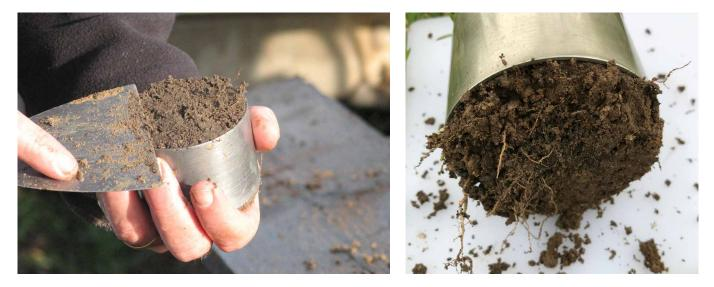
Figure 18. Collecting a soil sample to assess bulk density [Photos: Amanda Schapel].
