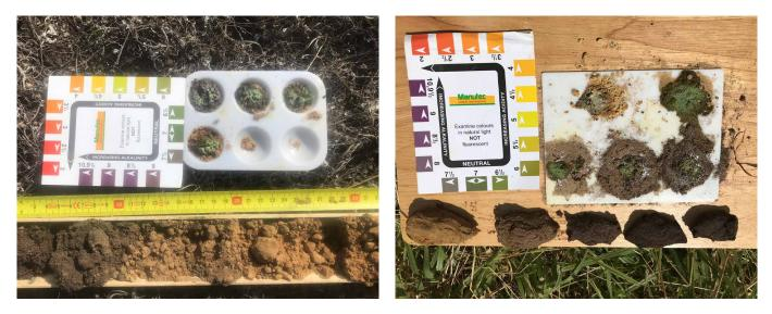
Figure 20. Using a field kit to assess soil pH [Photos: Amanda Schapel].
