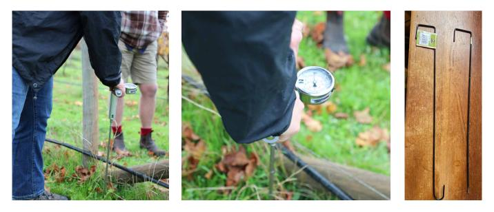
Figure 19. Soil penetrometer (left and middle) and a handmade penetrometer without pressure gauge (right) [Photos: Mary Retallack].
