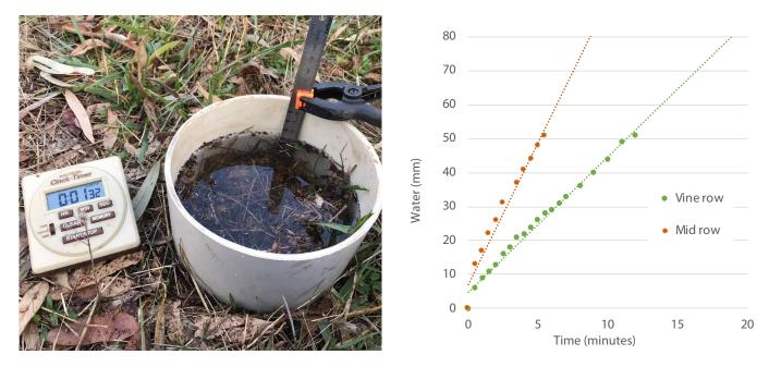
**Figure 16.** Water infiltrometer test and graphing the rate of water infiltration [Photo and Figure: Amanda Schapel].
