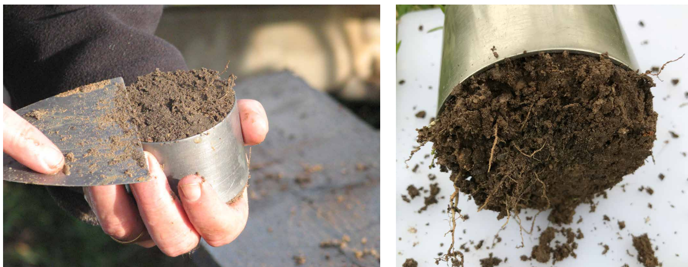
Figure 18. Collecting a soil sample to assess bulk density [Photos: Amanda Schapel].
