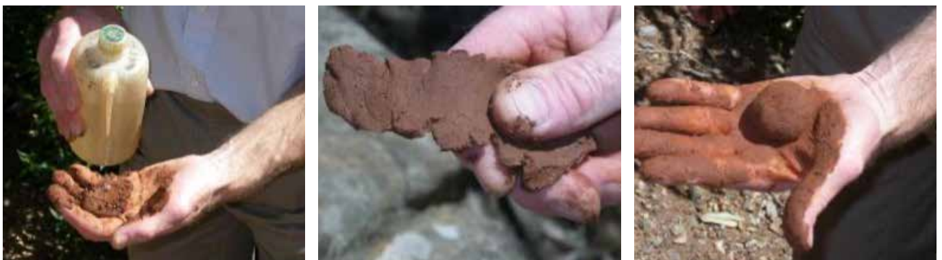
Figure 12. Hand texturing soil samples in the field [Photos: Maschmedt, 2004].
