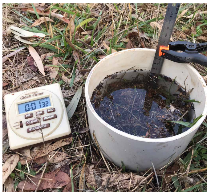
Figure 16. Water infiltrometer test and graphing the rate of water infiltration [Photo and Figure: Amanda Schapel].
