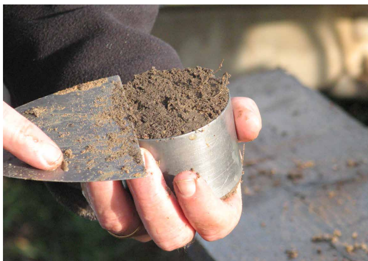
Figure 18. Collecting a soil sample to assess bulk density [Photos: Amanda Schapel].
