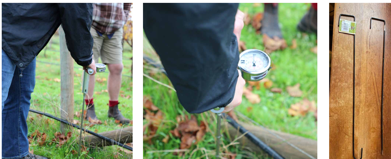
Figure 19. Soil penetrometer (left and middle) and a handmade penetrometer without pressure gauge (right) [Photos: Mary Retallack].
