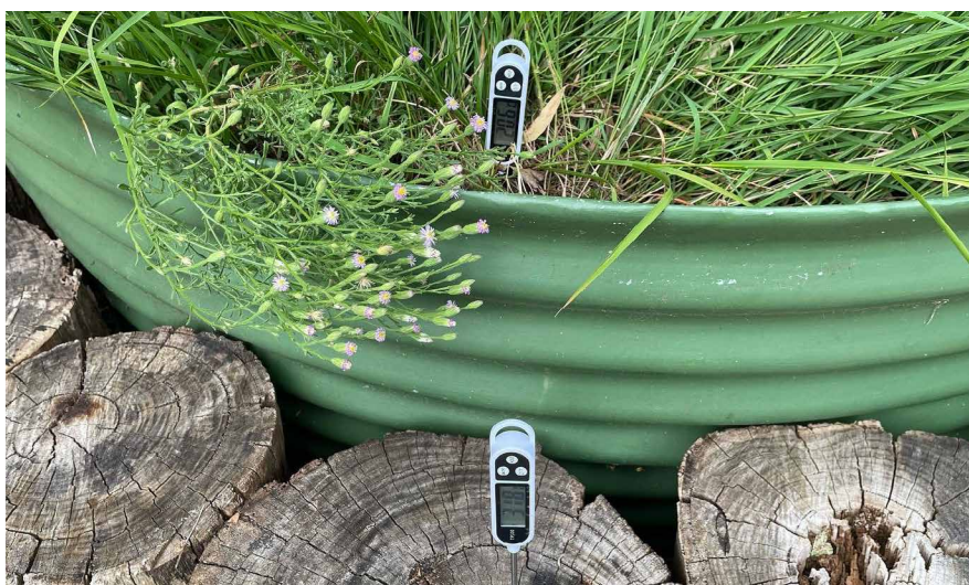
Figure 11. Measuring soil temperature in a vegetated versus ambient location [Photo: Mary Retallack].
