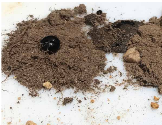
Figure 17. Water repellence test showing distinctive spherical droplet not penetrating soil (left), a paint pallet can be handy to keep samples separate when you are testing (right) [Photos: Amanda Schapel].
