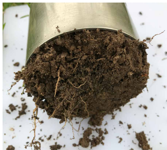
Figure 18. Collecting a soil sample to assess bulk density [Photos: Amanda Schapel].
