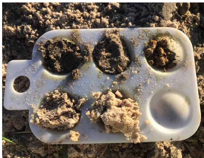
Figure 17. Water repellence test showing distinctive spherical droplet not penetrating soil (left), a paint pallet can be handy to keep samples separate when you are testing (right) [Photos: Amanda Schapel].
