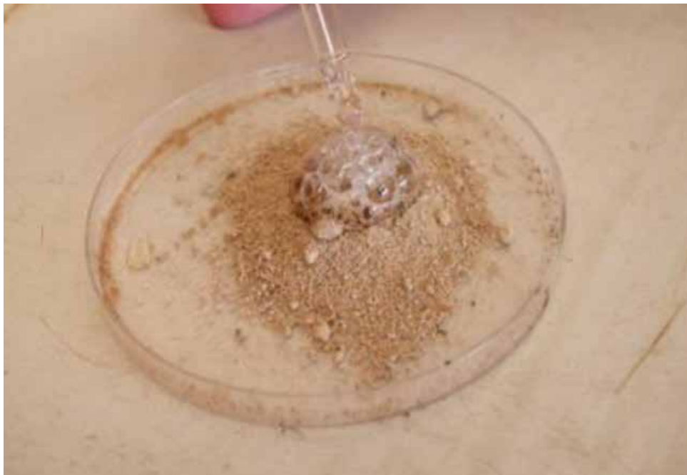
Figure 13. Example of a very high fizz reaction (Maschmedt, 2004).
