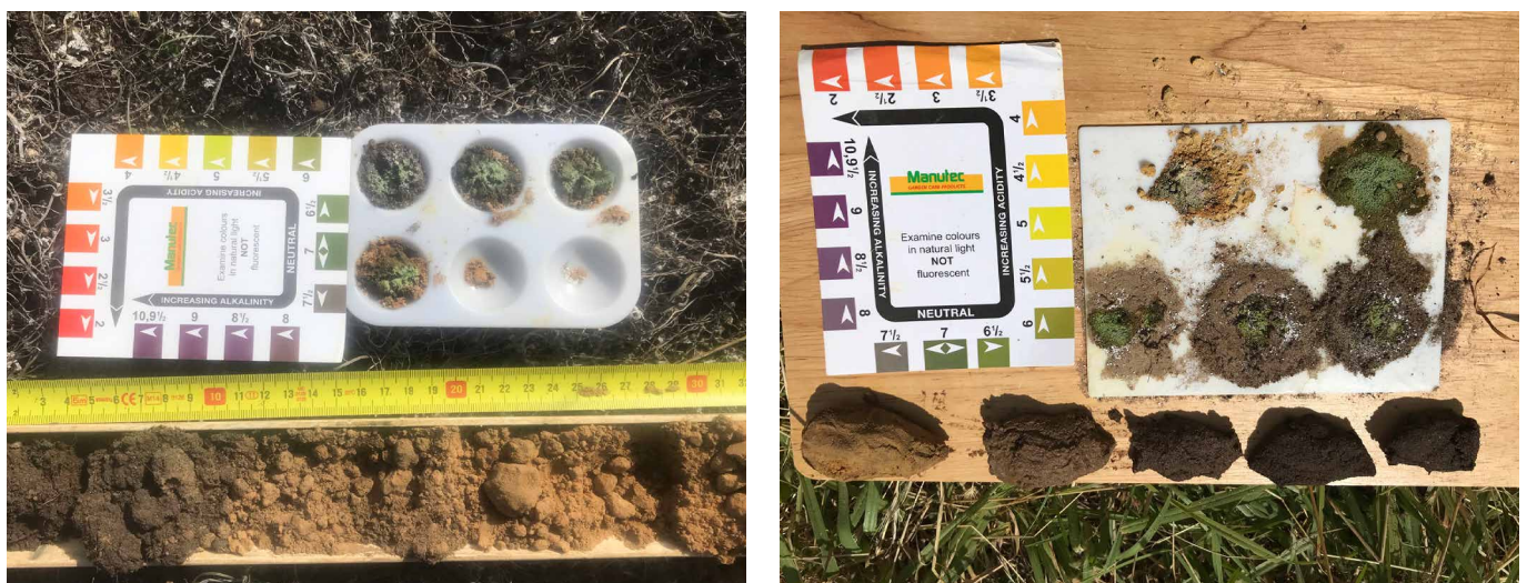
Figure 20. Using a field kit to assess soil pH [Photos: Amanda Schapel].
