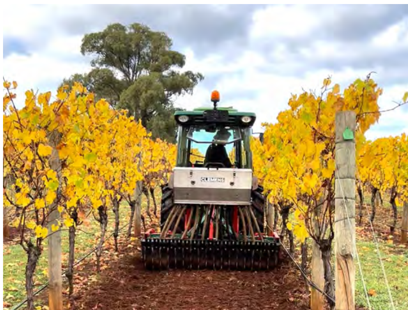
Figure 43. A rotary harrow fitted with a seed box (left) [Photo: Steve Faulkner], and power harrow without a seed box [Photo: Weekly Times].
