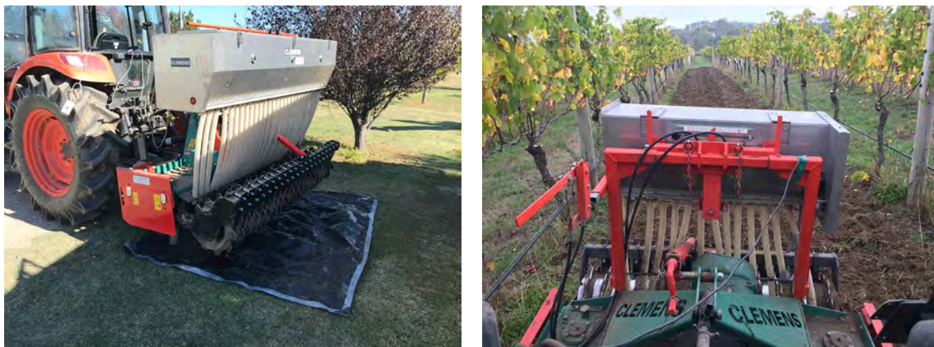
Figure 21. Calibrating a Clemens seeder (left) and in action (right), Mornington Peninsula, Victoria [Photos: Steve Faulkner].
