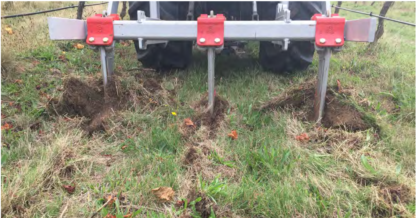
Figure 41. Tines (preferably offset) such as the Yeoman's plough can be used to open but not turn over the soil and break up hard pans prior to seed bed preparation [Photo: Steve Faulkner].
