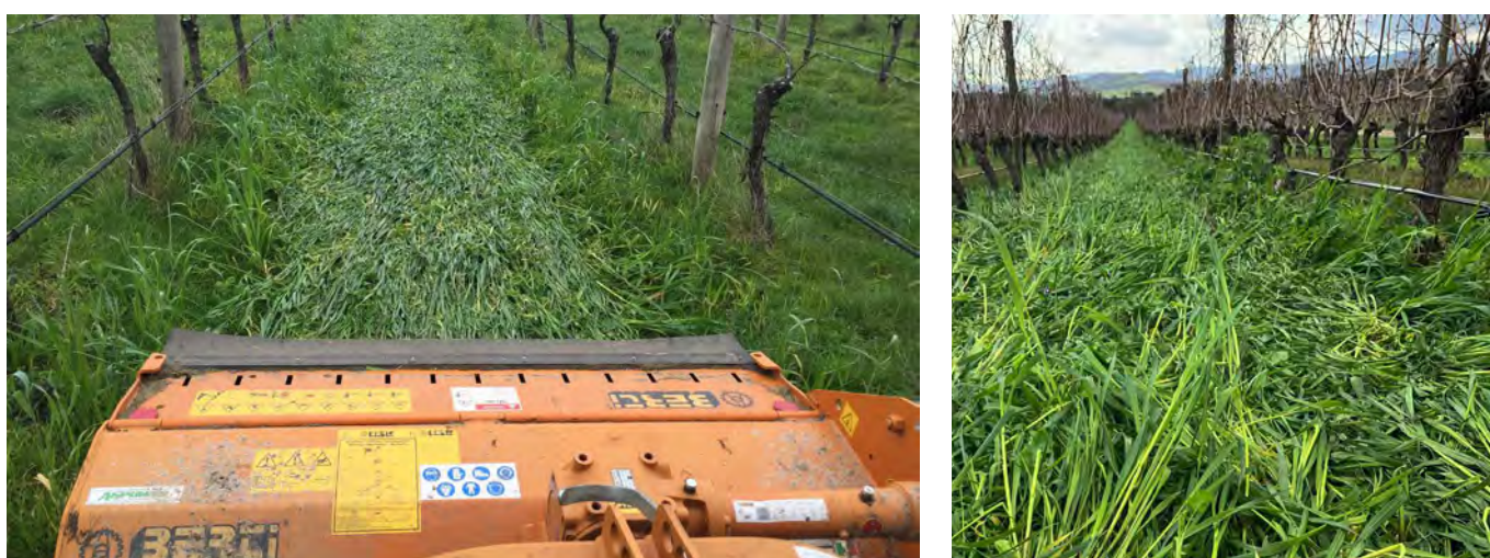
Figure 25. Rolling with a Berti mulcher that is turned off (left) and the resulting rolled cover crop in the midrow (right), Victoria [Photos: Steve Faulkner].
