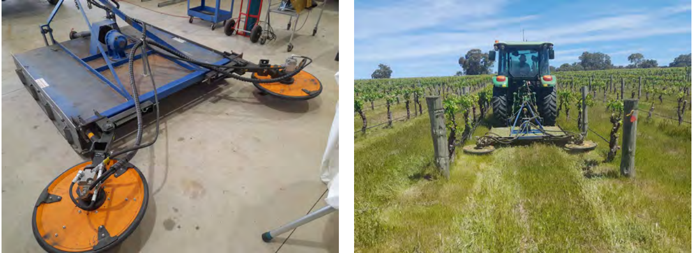
Figure 27. TMC Cancellia under-vine mower attached to a self-fabricated frame on the back of the mid-row slash, Eden Valley, South Australia [Photos: Dan Falkenberg].
