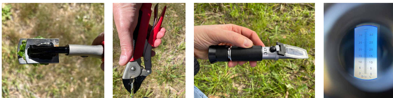
Figure 37. Leaf brix can be measured using a pair of modified vice grips to extract leaf sap and a refractometer which provides an objective measure of plant health [Photos: Mary Retallack].
